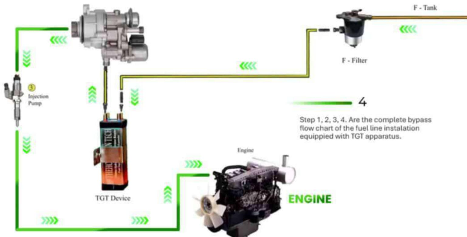
Step 1, 2, 3, 4. Are the complete bypass flow chart of the fuel line instalation equipped with TGT apparatus.
